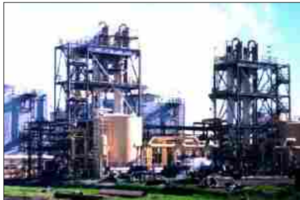
Figure 8: 4,600 m 2 self-cleaning heat exchanger surface replacing 24,000 m 2 conventional surface.
